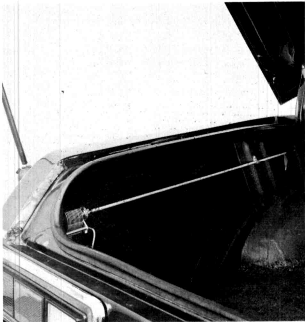
Tuning capacitor and limber shaft mounted in author's car. Planetary drive at capacitor prevents backlash and wind-up "hop" by reducing torque at capacitor.
